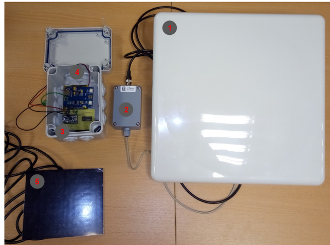
Fig. 1. The e-RFIDuino station and its five connected modules: RFID antenna (1), RFID SCIEL reader (2), Arduino datalogger, LiPo Rider, and batteries (3), housing box (4), and small solar panel (5).
