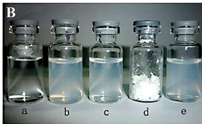
Fig. 5. (A) illustration of PTX micelles; (B) (a) normal saline (NS), (b) only micelles (blank), (c) MPEG-PCL/PTX micelles, (d) lyophilized powder of PTX micelles, and (e) re-dissolved freeze-dried PTX micelles. [Adopted and modified with permission from Wu et al.[165]].
