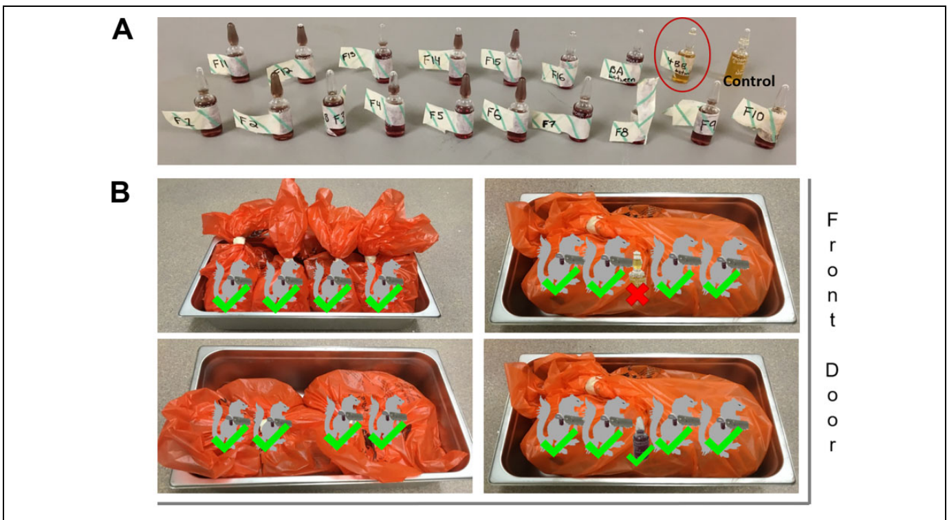
Figure 6. Results of ferret carcass test 1. (A) The biological indicator (BI) shown in the red circle failed the sterilization cycle. The control vial is shown at the top right. (B) The location of the failed BI is indicated.
