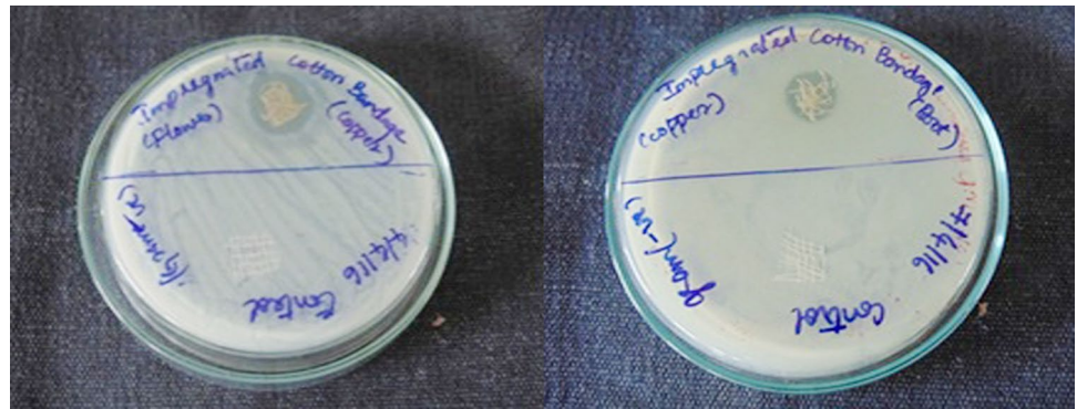
Fig. 14 Anti-bacterial activity of copper nanoparticles (flower and root extract) impregnated cotton bandage against E. coli , respectively
