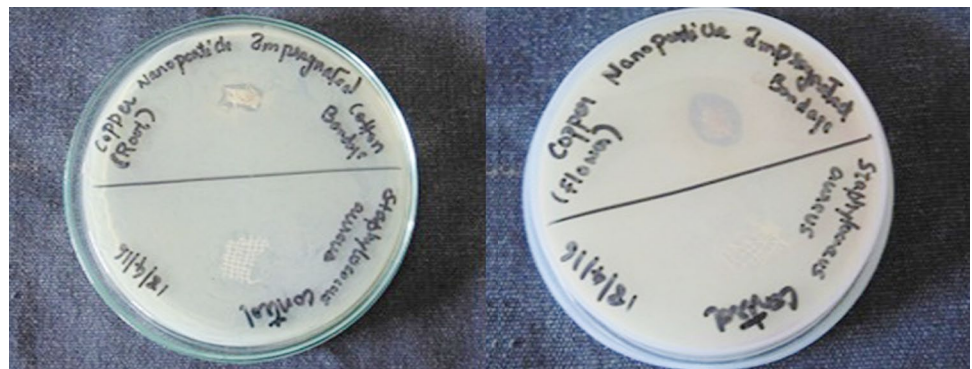
Fig. 16 Anti-bacterial activity of copper nanoparticles (root and flower extract) impregnated cotton bandage against S. aureus , respectively
