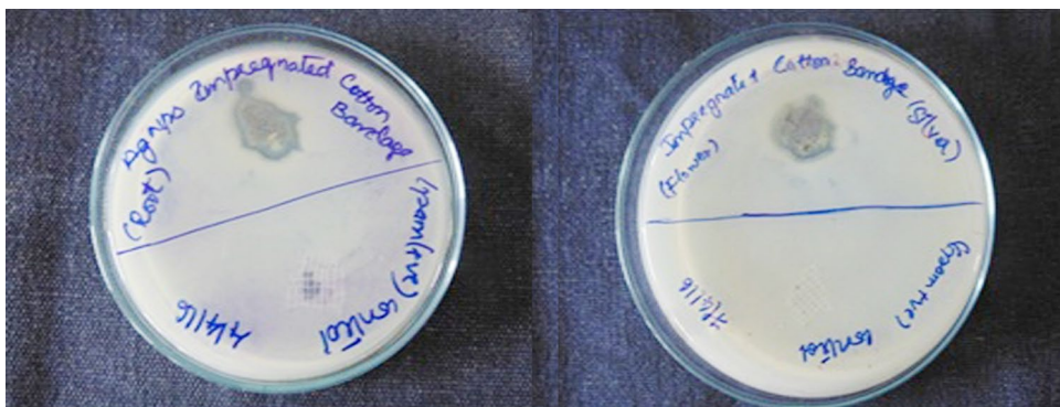
Fig. 13 Anti-bacterial activity of silver nanoparticles (root and flower extract) impregnated cotton bandage against B. cereus , respectively
