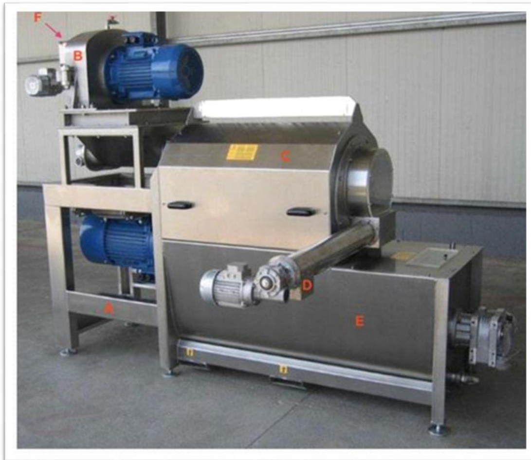
Figure 2. Partial destoner machine proposed by Romaniello, Leone and Tamborrino [16]. Legend: A: chassis; B: mechanical crusher; C: destoner; D: cochlea for pits extraction; E: malaxing; F: olive feeding.
