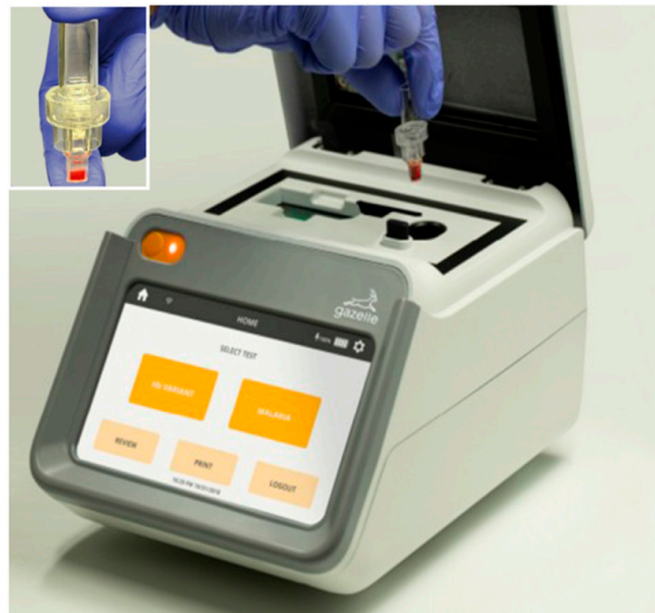
Figure 2. Cartridge loaded with blood sample at the time of insertion into the Gazelle™ device prior to hemozoin detection analysis. Image courtesy of Hemex Health.
