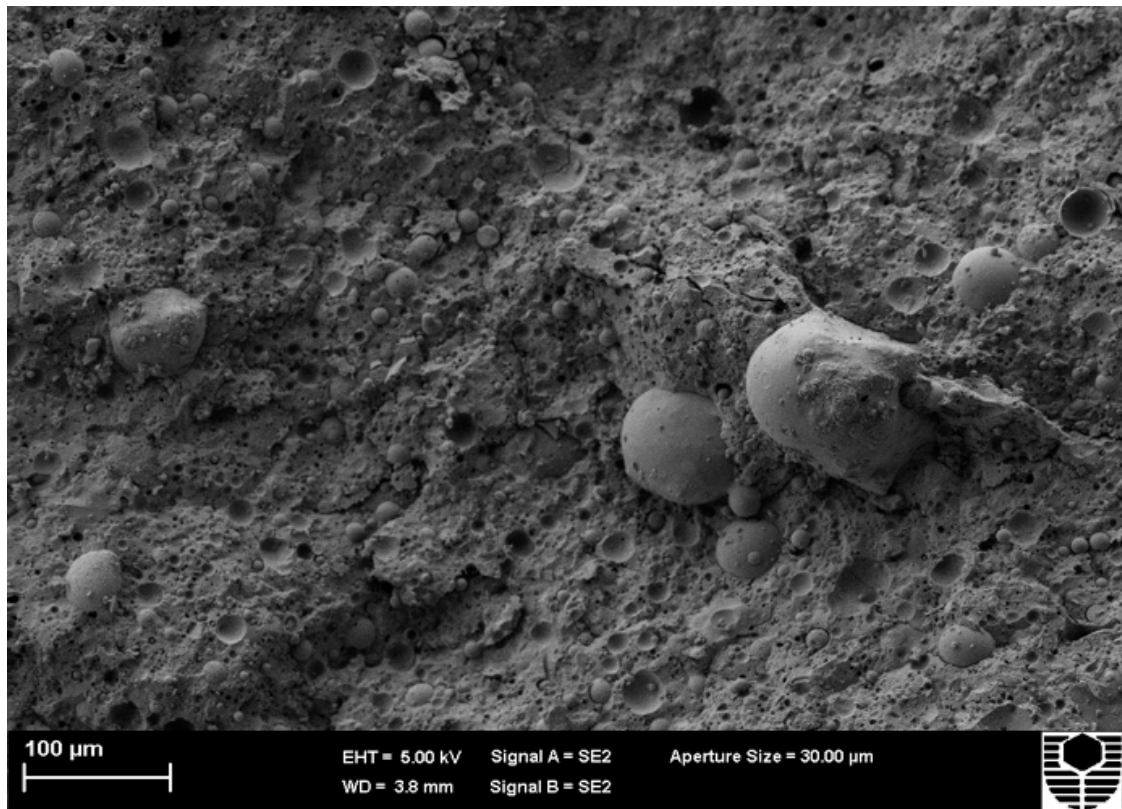
Figure 8. Microstructure of Mix 3 for FA-based geopolymer.
