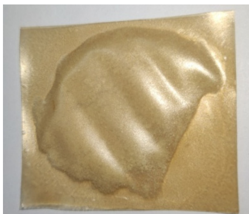
Figure 10. Application of \beta -glucanfilm with pomegranate juice for packaging powdered Vitamin C.
