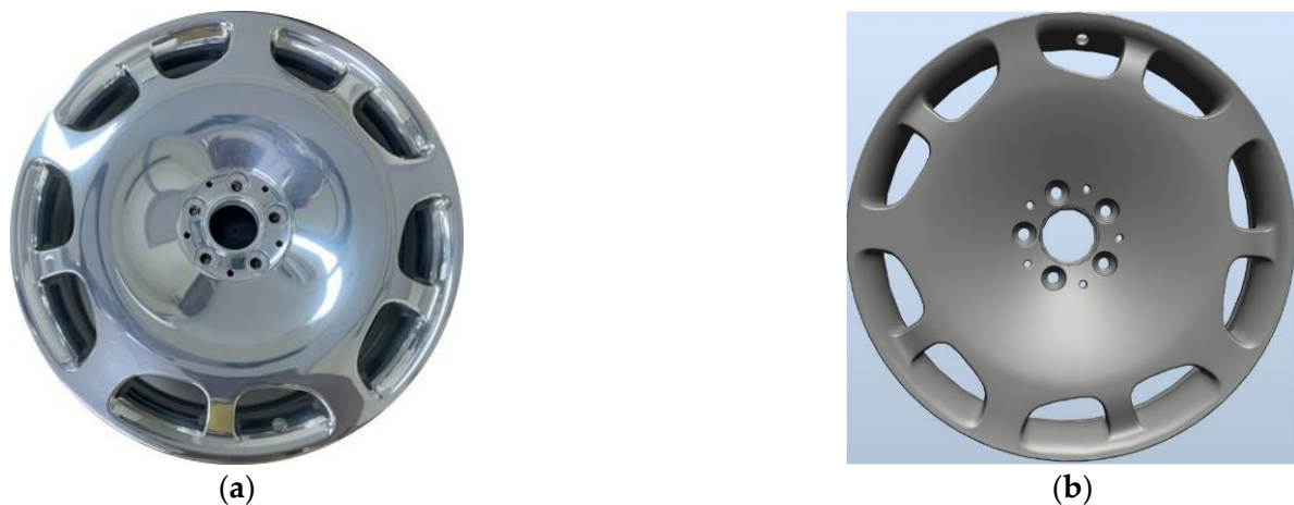
Figure 2. (a) Image of actual aluminum rim; (b) numerical rendering of the aluminum rim.
