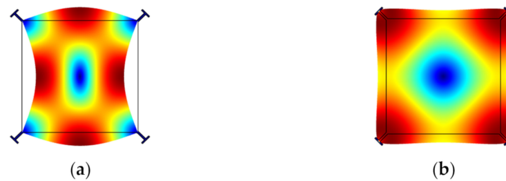
Figure 1. Finite element model (FEM) simulation of a BAW resonator with square plate structure in COMSOL. (a) WG mode; (b) Extensional mode.
