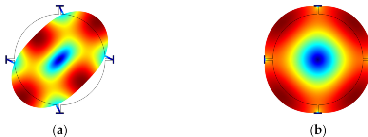
Figure 2. FEM simulation of a BAW resonator with disk structure in COMSOL. (a) WG mode; (b) Extensional mode.
