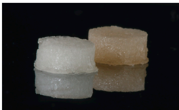
Figure 5. Visible-light photopolymerized NCHGs, the white does not contain drugs, and yellowish shows the CHX and Metr-filled hydrogel.
