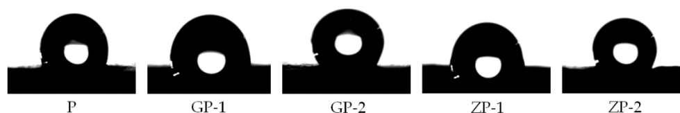
Figure 9. Water contact angle images of fabricated membranes.
