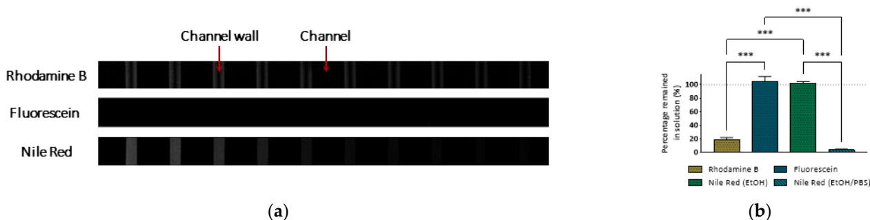
Figure 1. (a) Confocal microscopy images of PDMS channel walls following continuous flow of rhodamine B and fluorescein in 1\times PBS and Nile red in ethanol/PBS (1:3 v/v ). (b) Relative concentration ratio (expressed as a percentage) of 1\ \mu\text{M} rhodamine B, 1\ \mu\text{M} fluorescein, and 1\ \mu\text{M} Nile red in ethanol or ethanol/PBS (1:3 ratio) that remained in solution following 90 min of continuous flow through the PDMS microchannels at 96\ \mu\text{L}\cdot\text{h}^{-1} . Values show Mean \pm SD from at least three independent measurements (***) p < 0.001 .
