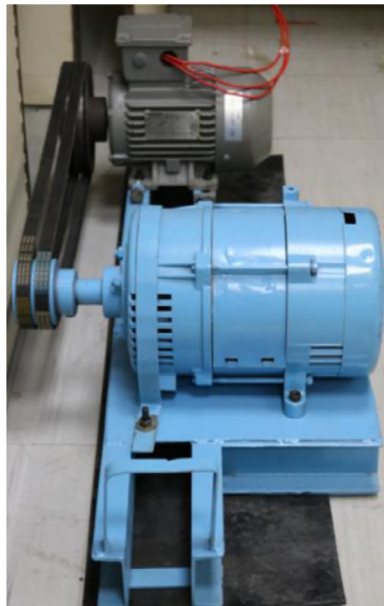
Fig. 1. Experimental setup for bearing fault diagnosis including a three phase motor and an alternator coupled through a belt.
