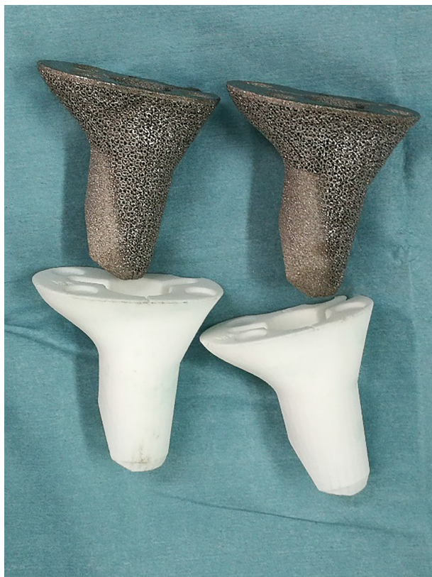
Fig. 1 Patient-customized three-dimensional (3D)-printed highly porous metaphyseal cones and their trials (Photograph courtesy: Dr. Yang Li, during the operation; we have the copyright of this image).
