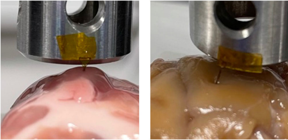
Figure 8. Insertion using Instron 5966 travelling at 1 \text{ mm s}^{-1} . Insertion was successful in deeper regions of the brain tissue, and unsuccessful when attempted through the pia mater. (Online version in colour.)
