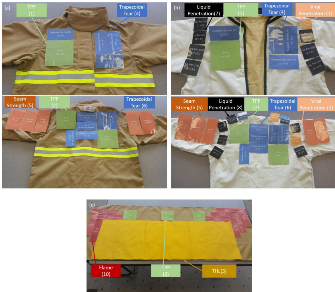
Figure 2. (a) Shell specimen locations at the front (top) and back (bottom). TPP (3), Tear (Warp, 5; Fill, 5), Seams (5); (b) Moisture barrier and thermal liner specimen locations at the front (top) and back (bottom). TPP(3), Tear (Warp, 5; Fill, 5), Seams(5). For moisture barrier only Liquid Penetration (15), Viral Penetration (3); (c) Blanket specimen locations at the front (top) and back (bottom). All three layers - TPP(3), THL (3). For shell only Flame (Warp, 5; Fill, 5).
