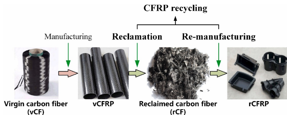
Figure 3. Recycling Process from Virgin Carbon Fiber to CFRP.
