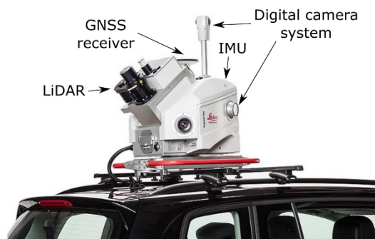
Figure 1. An example of an MMS: a vehicle-mounted mobile mapping platform consisting of different positioning and data collection sensors to generate an accurate georeferenced 3D map of the environment. Shown here are the main sensors of the Leica Pegasus: Two Ultimate as an example. Photo courtesy of Leica Geosystems [13].
