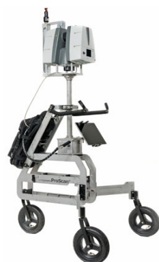
Figure 4. Leica ProScan trolley-based MMSs. Photo courtesy of Leica Geosystems [13].
