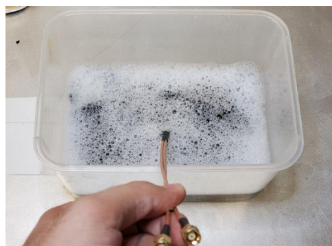
Figure 11. The fabric is completely submerged in water and detergent. The SMA connectors are held outside.
