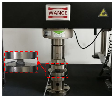
Figure 2. Testing machine for external calibration.
