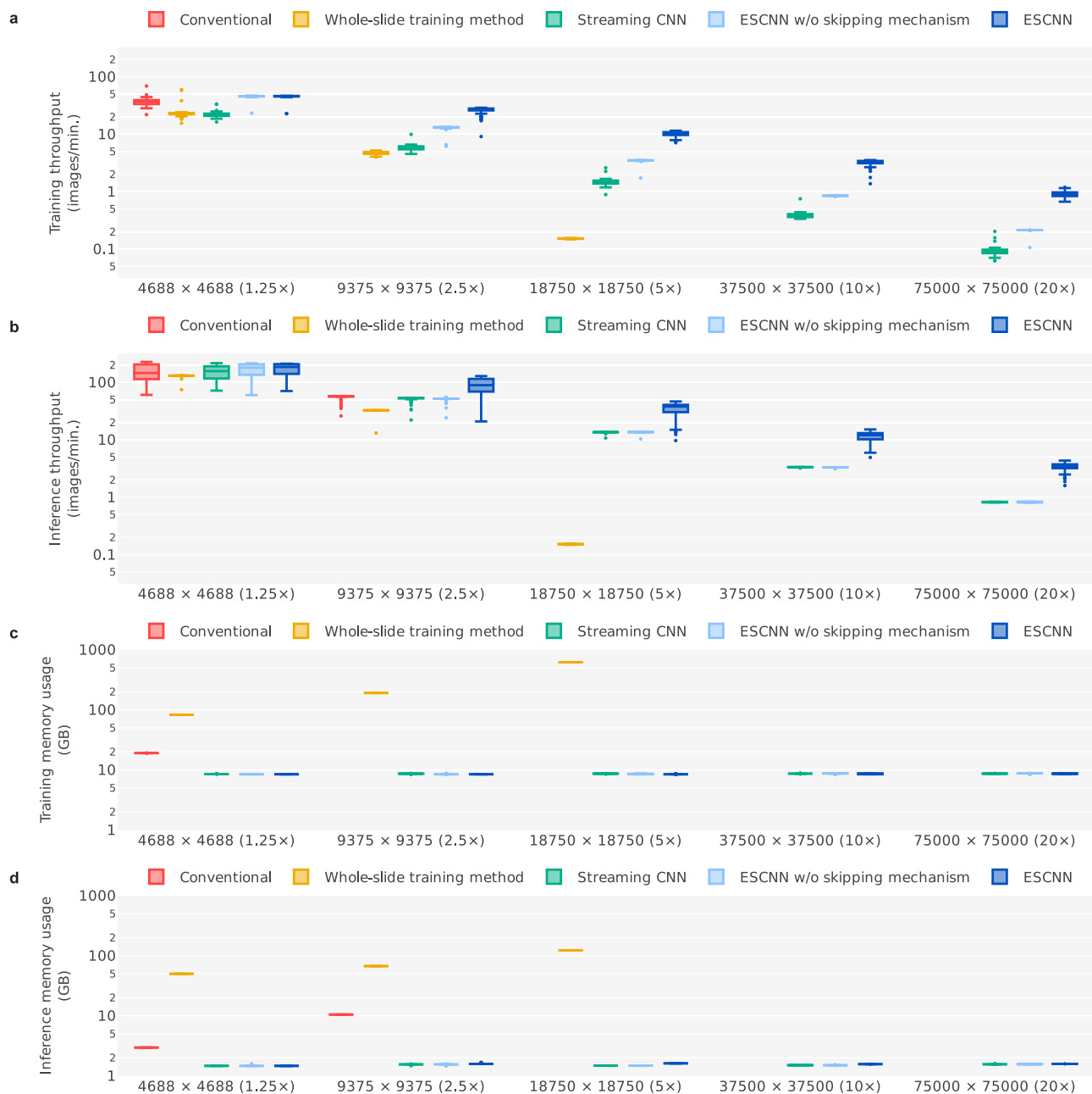
Fig. 3 Throughput and memory consumption of end-to-end training methods under various magnification levels of LN images. Each panel represents the (a) training throughput, (b) inference throughput, (c) training memory consumption (referring to Unified Memory for the whole-slide training method and GPU memory for the others), and (d) inference memory consumption. For each setting, we recorded the training/inference time and memory consumption when processing each LN image ( n = 100 images in total, sampled from the main training set). Each box-and-whisker plot comprises the center (median), the bounds of boxes (Q1 and Q3), the bounds of whiskers (the minimum and maximum within the range, obtained by adding the median to \pm 1.5 times the Q3–Q1 distance), and the outliers of the underlying 100 samples. The absence of certain boxes indicates that those settings could not be run due to memory shortages.
