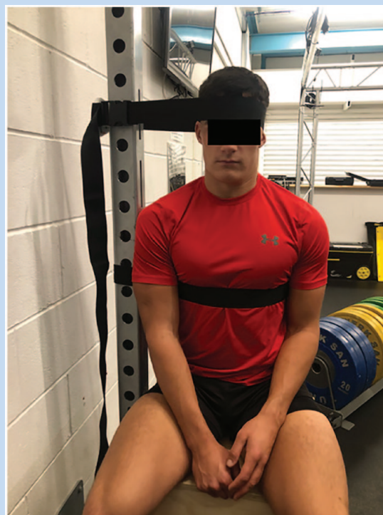
Figure 3. Example of player and equipment positioning during maximal voluntary isometric contraction testing during neck left side flexion.
