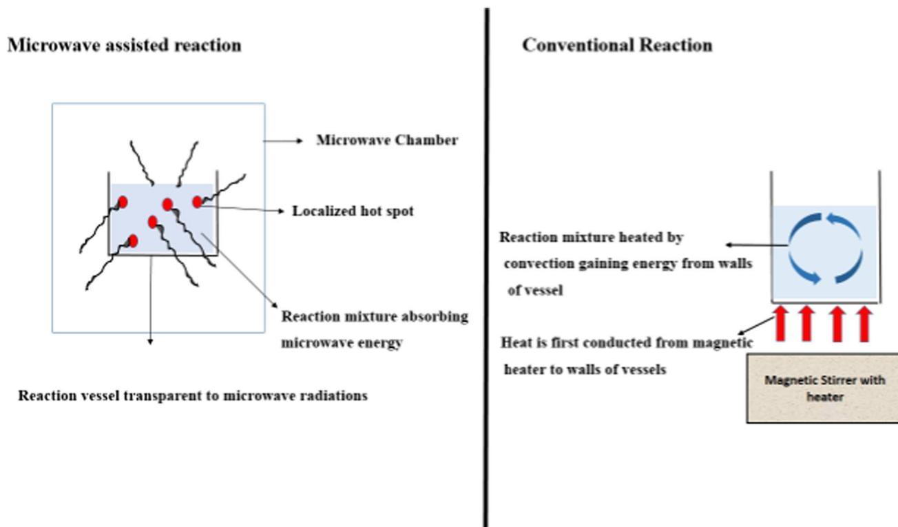
**Fig. 3** Figure representing comparison between microwave and conventional reaction
