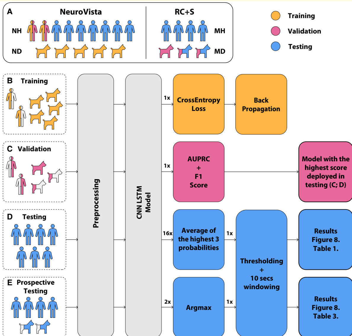
Figure 2 Schema of training, validation and testing data sets used in development of a generic, automated seizure detection algorithm for canines and humans. The preprocessing pipeline is the same for all data sets and represents the transition from raw iEEG data to normalized spectrograms. (A) Retrospective data included human and canine data sets acquired with two different investigational devices, NeuroVista (NV) and RC + S TM device. (B) Algorithm training was performed using retrospective data from humans and canines collected with NV devices. (C) The validation data included NV data from two humans (NH1 and NH2) and RC + S TM data from three canines (MD1–3). The validation data set was used to select the optimal convolutional neural network with long-short-term memory (CNN LSTM) model that was subsequently deployed in testing. The area under the precision-recall curve (AUPRC) and F1 score was calculated on the validation data set during training. The model with the highest combined score was deployed in testing. (D) Pseudo-prospective (data from seven humans; NH3–9) and (E) prospective (RC + S TM data from four patients MH1–4 and two pet dogs MD2 and MD3) ambulatory testing in human and canines living in natural environments (human at home and dogs living with their owners) were performed over multiple months (see results in Fig. 8 and Table 3). To get one probability signal from NV and RC + S TM devices, we aggregate CNN LSTM model outputs from multiple channels by average and argmax functions, respectively.
