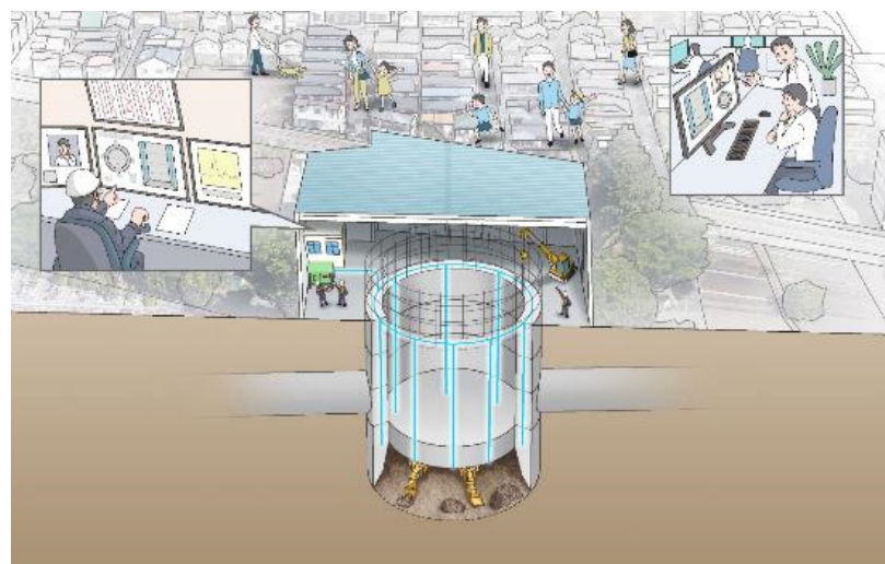
Figure 10. Example of open-type caisson during construction.
