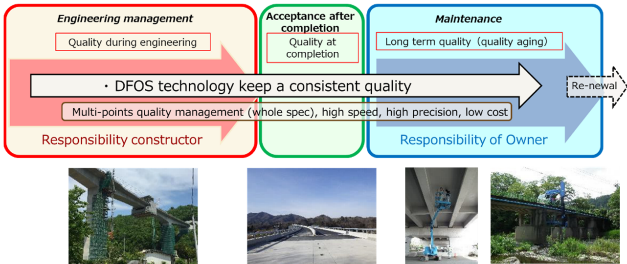
Figure 1. DFOS is a technology for the entire life cycle of a structure's monitoring.
