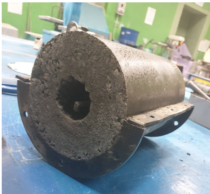
Figure 3. General view of the vibrocentrifuged prototype of the annular section.
