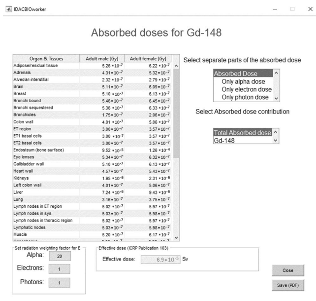
FIG. 6. The graphical interface of the result from the software with the continuous intake of 1 Bq per day of ^{148}\text{Gd} during 10 year.
