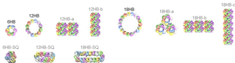
Fig. 4 Representative models for the 6HB, 12HB, and 18HB structures used for calculating CCS values reported in Table 1. Multiple 6HB barrels are either placed side-by-side (12HB-a, 18HB-a, and 18HB-b) or stacked end-to-end (12HB-b and 18HB-c). The larger-diameter barrels 12HB and 18HB, next to 6HB, are also compacted laterally to generate the flattened and “squished” models 6HB-SQ, 12HB-SQ, and 18HB-SQ.
