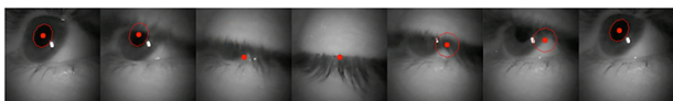
FIGURE 1. Example of a true blink (TB; i.e., a blink that was recorded by the software and occurred in the visual inspection [VI] at the same time). This example is from the Pupil Core device. The ellipse around the pupil disappears when the pupil is more than 50% covered, and this event is counted as an eye blink.
