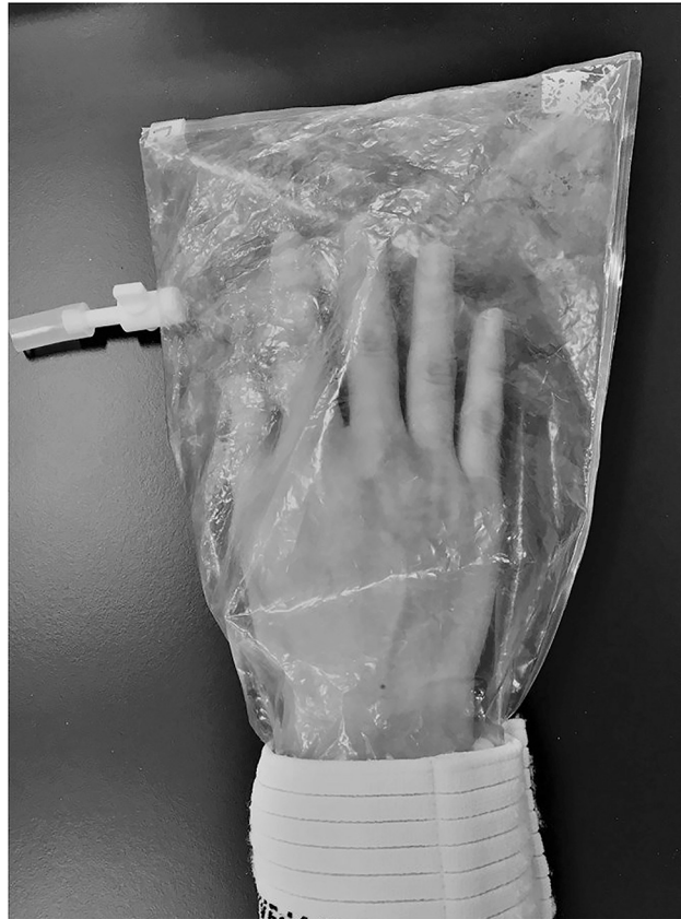
Fig 2. Collection bag for skin gas emanating from subjects' hands. Hands washed with unscented soap were covered with sampling bags made from a fluorinated ethylene-propylene copolymer material. The air inside was replaced with nitrogen and recovered after a certain period.
