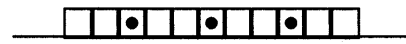
Figure 1. k = 3 mismatching characters (denoted by filled circles) distributed equally over a repeat of length l = 11 , yielding a minimum seed size of
