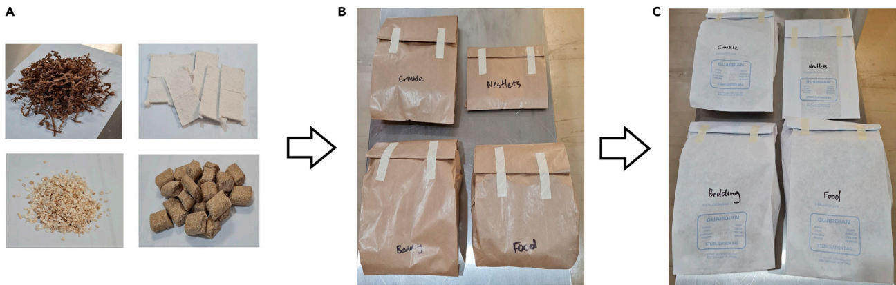
Figure 3. Order of packing sterile supplies into paper bags (A–C) Consumables (A) are packed firstly into brown paper bags (B) followed by white autoclave bags (C).
