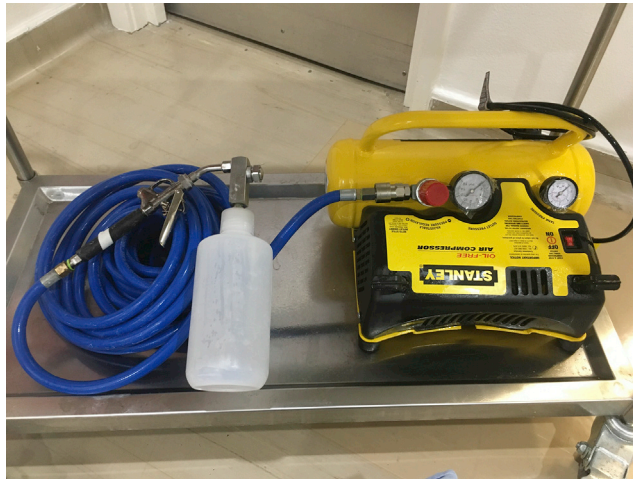
Figure 2. Sprayer Less atomizer unit which must be coupled by hose to an air compressor to operate
