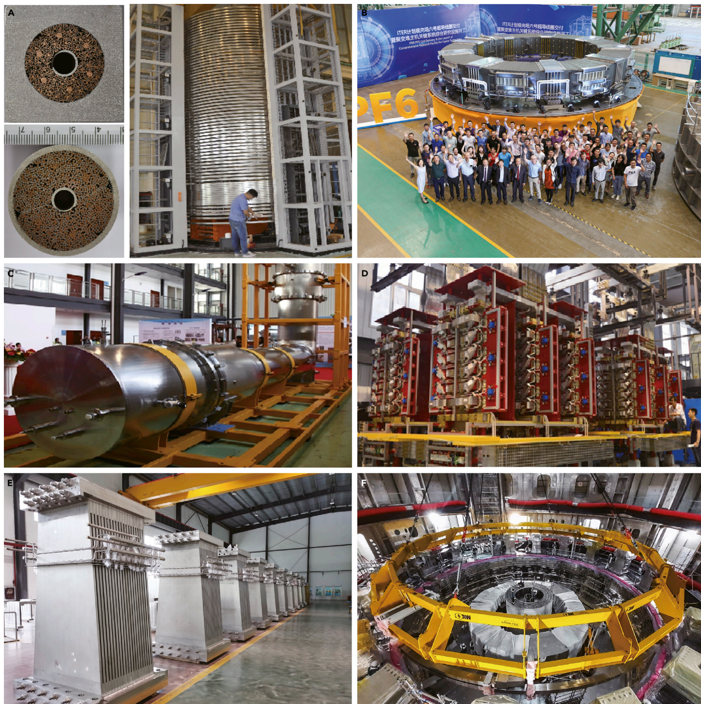
Figure 6. Progress of ITER activities in China (A) ITER CICC conductors. (B) ITER PF6 coil. (C) ITER feeder. (D) ITER AC/DC converter system. (E) ITER TFGSs. (F) ITER magnet support site assembly.
