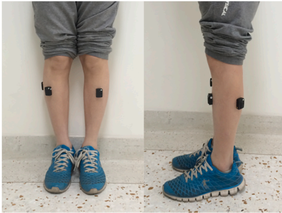
Fig. 2. sEMG Sensor and Electrode Placement [73].
