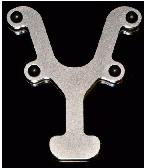
Figure 2. Metal reference guide with the four steel spheres inserted.
