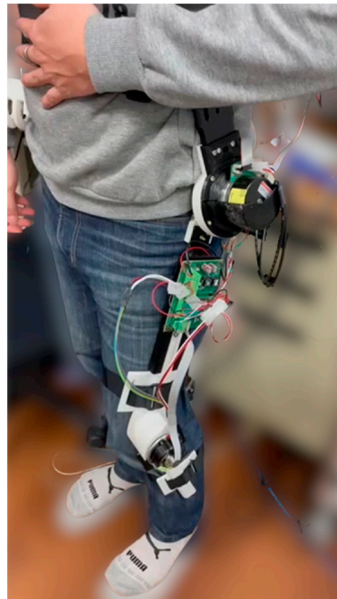
Figure 6. A subject wearing the robotic hip-knee exoskeleton.
