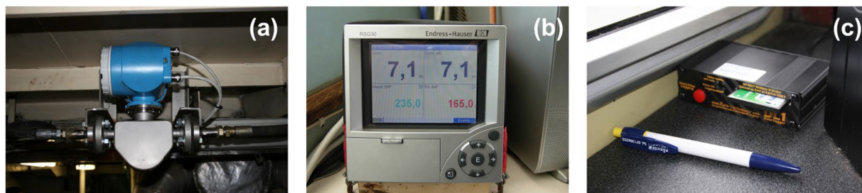
Fig. 2 Engine fuel efficiency system mounted onboard the monitored fishing vessels. (a) mass flow sensors for fuel consumption measurement; (b) multi-channel recorder mounted on the vessel's bridge to visualise the fuel consumption; (c) GPS data logger.
