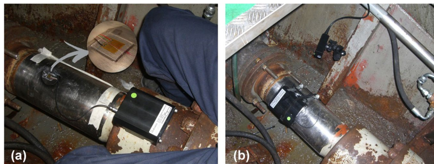
Fig. 4 Torque meter and video camera RPM counting device. Both apparatuses are used for the shaft power evaluation: (a) magnifier glass showing the strain gauge installed on the propeller shaft and connected to the data acquisition box; (b) video camera used to transmit the torque and rotational speed to a personal computer by an RS232/485 serial port.
