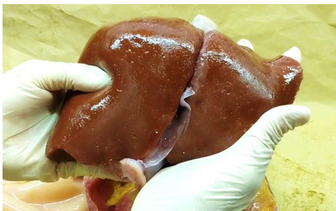
Figure 3 The final prototype organ model features all the internal anatomy shown in figure 1, modified additive manufactured using the materials and methods discussed previously. The prototype surrogate organ demonstrated characteristic softness and slumping characteristics of the real organ when handled. Slumping and relaxation of the soft tissue were reflective of the real organ especially during delivery and transposition of the organ and during palpation.
