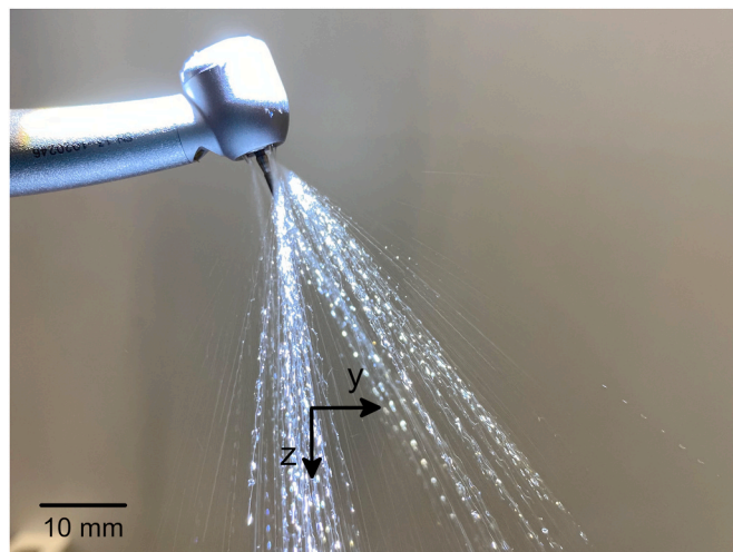
Fig. 7. The formation of droplets at the tip of the KaVo Expert Torque™. The arrows showing z and y directions point towards the positive directions. The positive values of the x direction are pointing away from the reader. The origin point was at 3 cm below the tip of the dental instrument as illustrated on the figure.
