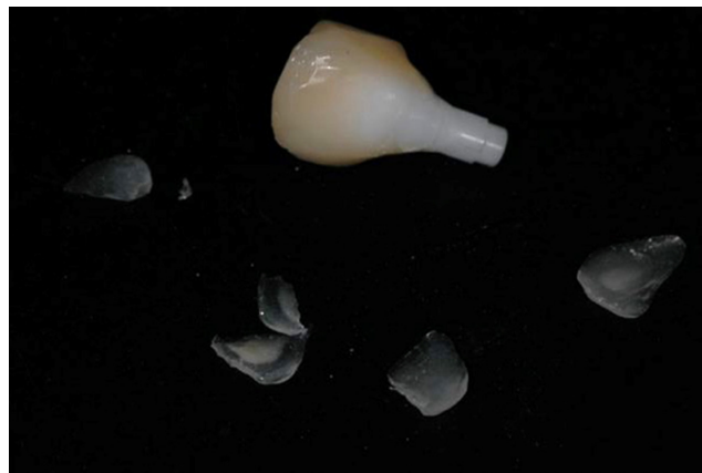
FIGURE 1 Multiple chipping of the veneering ceramic at a zirconia-based implant single crown
