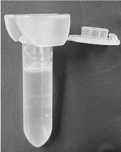
Figure 6. 70 µm filtration setup
