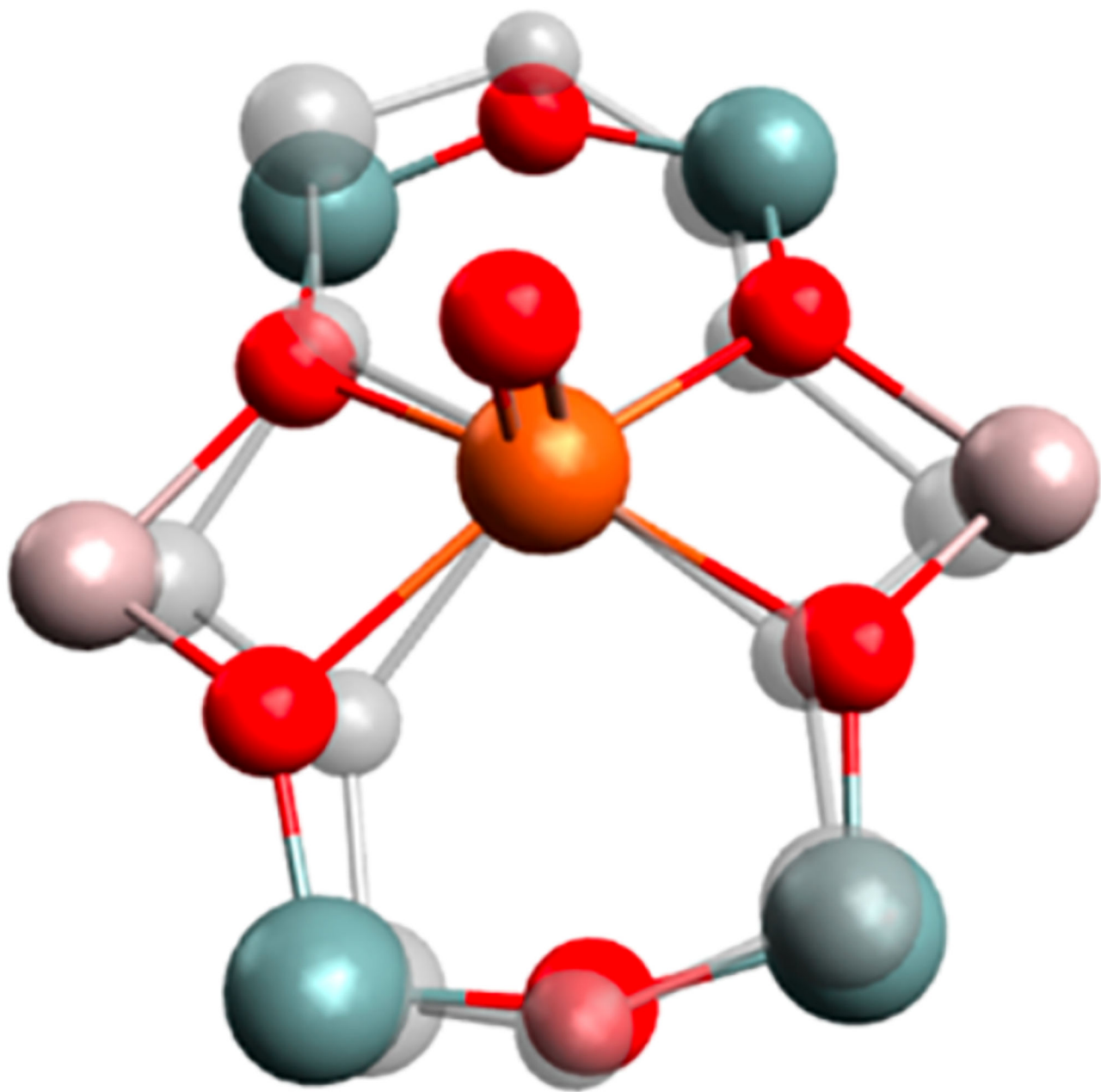
Figure 40. DFT optimized structural overlay of the \alpha -O site that forms in the *BEA lattice (grey) and the CHA lattice (colored). (Color scale: red: O; pink: Al; grey: Si, and orange: Fe.) Reproduced from ref 71. Copyright 2018 American Chemical Society.
