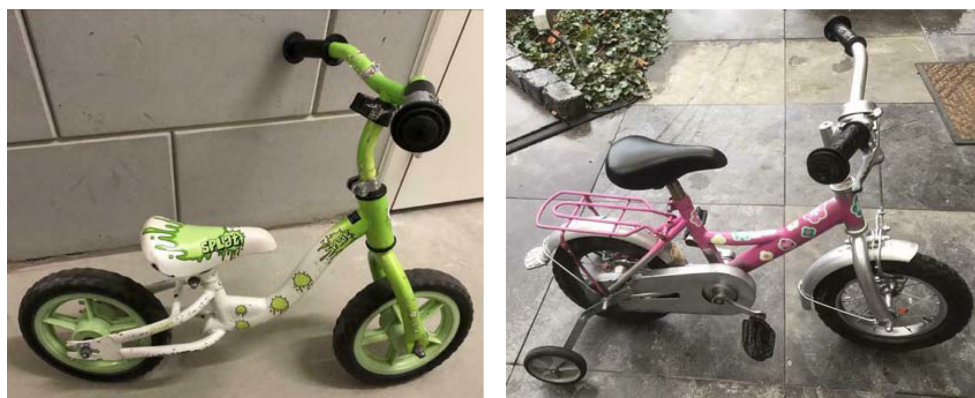
FIGURE 1 A balance or runner bicycle (left) and a bicycle with training or support wheels (right)
