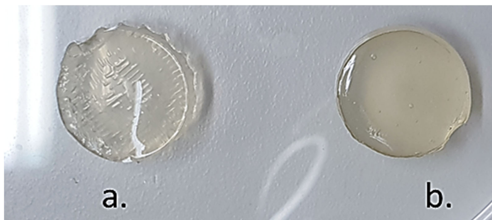
Figure 9. Images of typical 3D printed SA-GL tablet-shaped matrices produced using a 3D bioplotter in the least and most favorable concentrations: (a) Least favorable printing ink (5%SA-8%GL) and (b) Most accurate printing ink (8%SA-10%GL).
