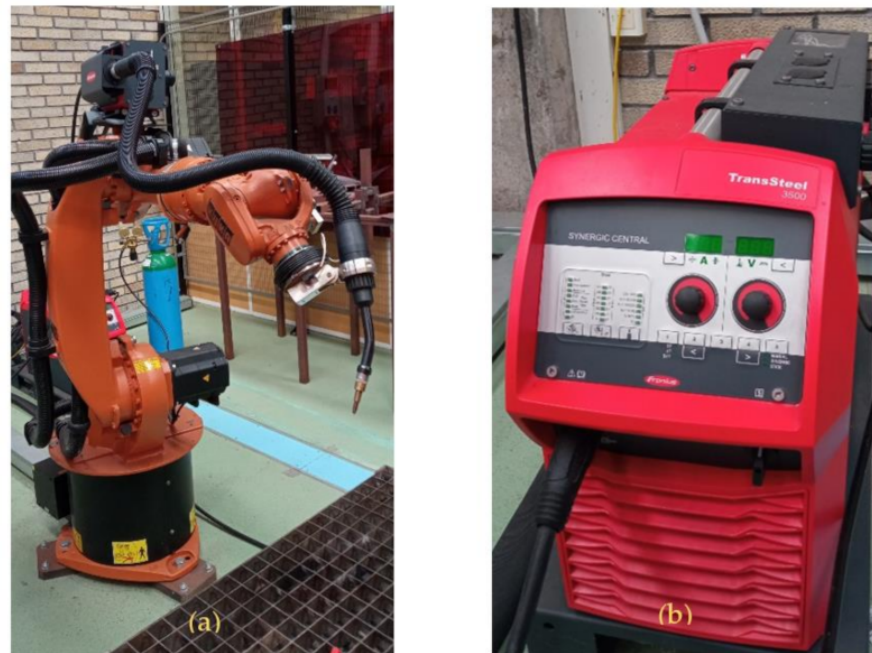
Figure 2. (a) Robot KUKA Kr 16, Torch and wire feed motor, (b) Fronius power generator Transteel 3500.
