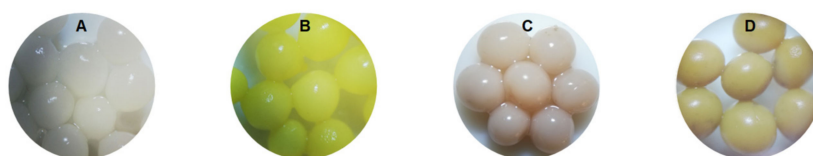
Figure 1. Photographs of synthesized biosorbents ((A,B)—SPA 5%; (C,D)—SPRBA 5%) before (A,C) and after (B,D) biosorption of ethacridine lactate.
