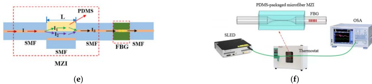
Figure 1. (a) Schematic diagram of the dislocation fiber MZI-based sensor [48]. (b) Schematic of HBEF sensor based on a Sagnac loop [51]. (c) Schematic diagram of an SI based on a PMF with a circle [53]. (d) Diagrammatic sketch of the PDMS-coated microfiber sensors [60]. (e) The sensing probe with cascaded MZI and FBG [62]. (f) Schematic of temperature measurement system [63].
