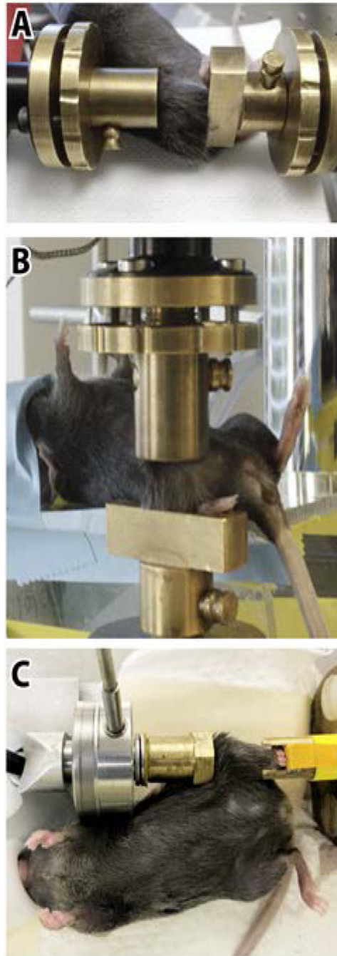
Figure 2: Photos of different loading devices used to perform in vivo tibial loading in mice 42; 63; 80; 100. A and C show mice in supine position with a horizontally-oriented tibia. B shows a supine mouse with vertical tibial orientation.
