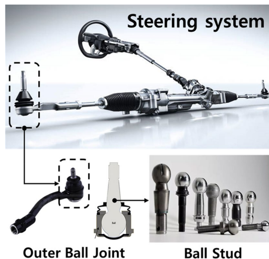
Figure 1. Ball stud parts of a steering system 7–10 .
